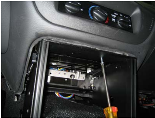
Attach using #10 x 3/4" sheet metal screws.
